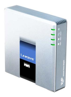
Two standard telephone ports for analog phones or use one of the ports for a fax machine, each with an independent phone number
