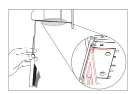
If your VC500 codec cannot be mounted on the top of a TV when the bracket has reached the edge of the VC500 codec, choose other installation methods. The VC500 codec may fall down when the thickness of the TV is more than 77 mm. In this situation, do not mount the VC500 on the top of a TV.
