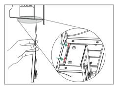
If your VC500 codec cannot be mounted on the top of a TV when the bracket has reached the given location, you should remove the bracket, and then convert its direction. Refer to the following section for more information.
