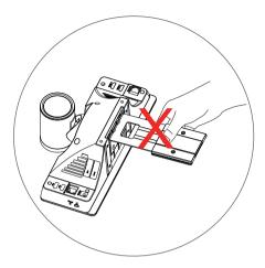
Do not pick up the bracket which connects with a VC500 codec, the VC500 codec may fall down in this situation.
