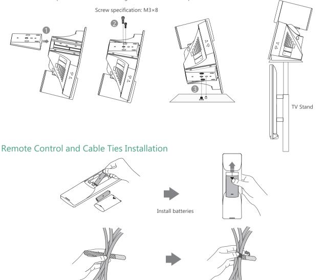
Fasten the cables with the cable tie
