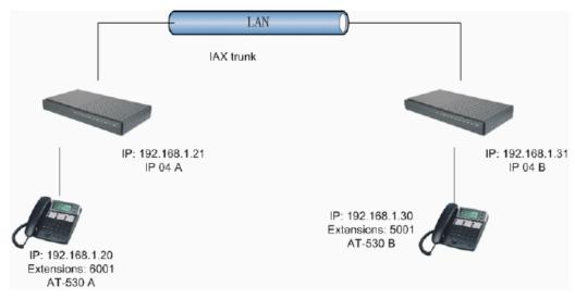
Below is the structure of how to link two IP04s in the same LAN:
