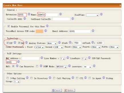
Use the same method to add the extensions: 6002, 6003 and 6004. In our system picture, we use softphone x-lite to register on 6001 and 6002. Use AT-530 IP phone to register on the extensions 6003 and 6004. Then these four extensions can communicate with each other use the numbers 6001, 6002, 6003 and 6004.
