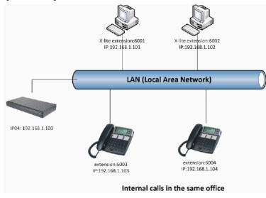
At the beginning, we need to add some extensions to make internal calls. Each extension acts as an internal number. There are three types of extensions we can add: SIP, IAX2 and ZAP.
