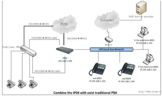
1/ Connect the FXO port of the PABX to IP04's FXS port. so the PABX will be one of the IP04's FXS extensions and all the extensions under pabx can use all the fxs functions from IP04, the functions include:
