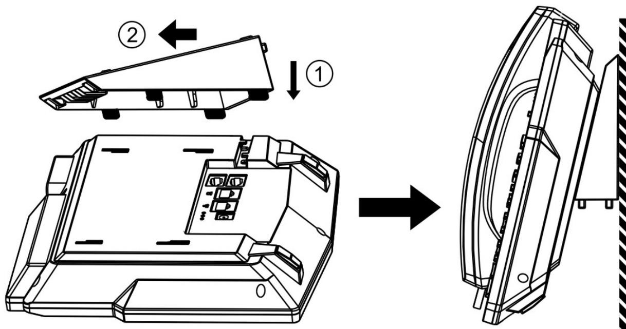
**Figure 3 - Wall-mount Installation**
