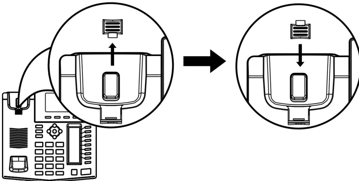
Figure 2 - Change handset hook to wall-mount mode
