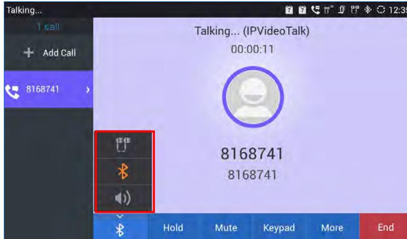
Figure 56: Switch Audio Channel during Call 2
