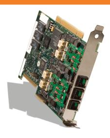
PIKA for Asterisk Low Density Analog Boards with DSP based echo cancellation plug-in to computer systems to connect your applications to both TDM and IP networks. They are a 4-port, half-length boards with a PCI interface that supports the new universal 3.3 volt power bus.
