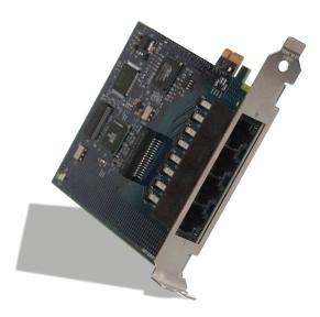
PIKA for Asterisk T1/E1 Gateway Boards with echo cancellation feature market leading flexible port densities. Currently available in a PCI variant with PCIe coming later this year. Up to four T1/E1 network interfaces can be enabled with in field license upgrades.
