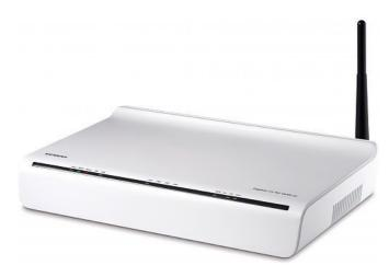
Introducing the Siemens SX762 all-in-one integrated phone and network system. This small but powerful box forms the heart of a small or home office communication system. This single low cost device provides Internet access, telephone IP-PBX system for up to six phones, four port network switch, file and print server capabilities and wireless networking.
