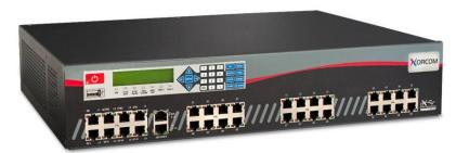
or E1 R2 ports in a single, 19" 2U chassis. Additional PSTN/analog phone ports can be provided by connecting external <u>Astribank</u> units via the USB2 ports, for a total of up to 672 PSTN/analog phones ports, up to 1000 users and up to 480 concurrent calls.
