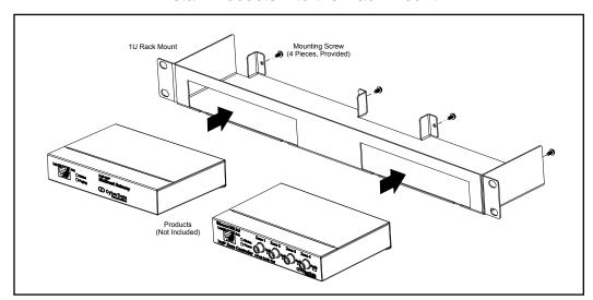
Install the Rack Mount into the Server Rack
