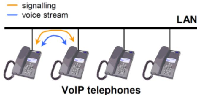
**Figure 3.31:** "Point-to-Point" Arrangement
