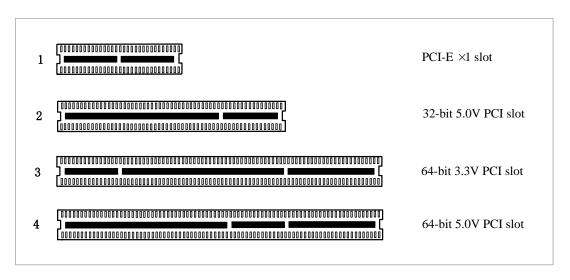
Figure 2 PCI-E and PCI slots
