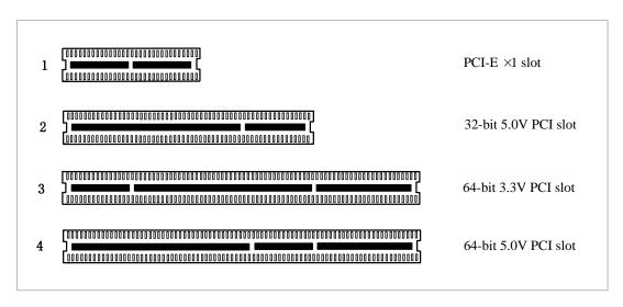
Figure 2 PCI-E and PCI slot
