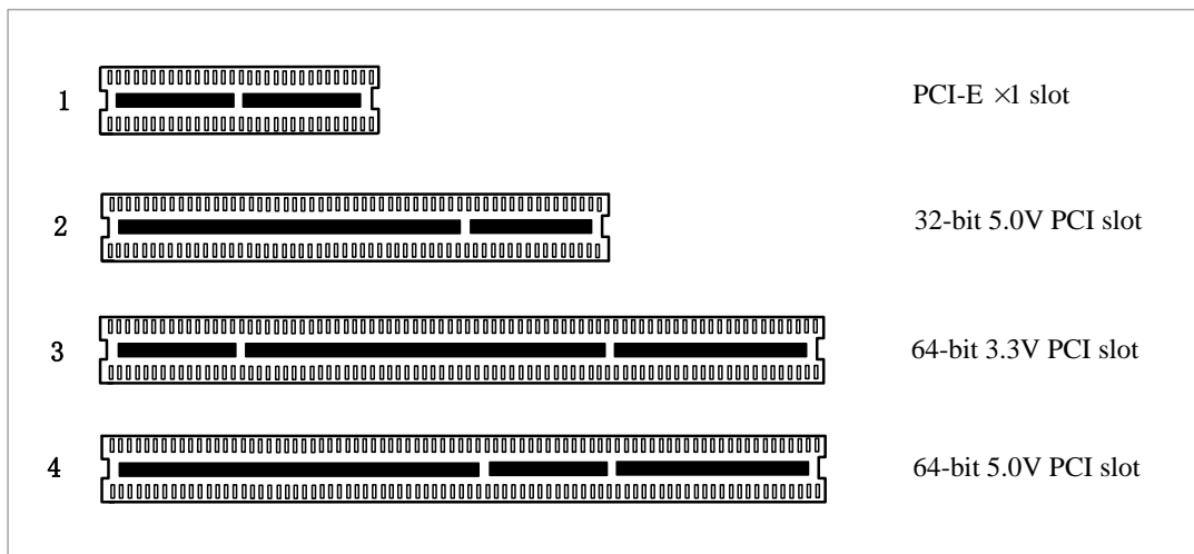
Figure 2 PCI-E and PCI slot
