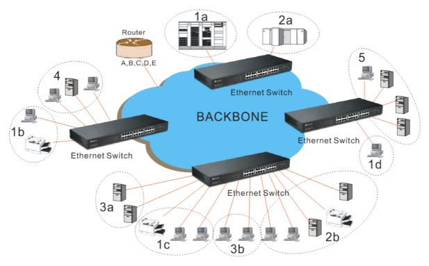
Now we apply VLAN technology to configure the system shown as the figure above. We can partition the users into the different logical networks which have their own broadcast domain. The traffic will not disturb among these logical networks. The users 1x (x denotes  $a \sim d$ ) are members of VLAN 1. Any traffic within VLAN 1 does not flow to VLAN 2 and
