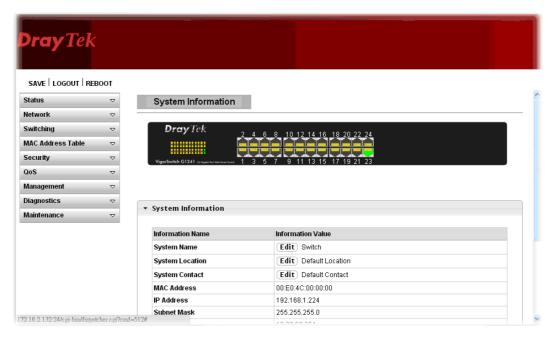
First, IP Address: as shown above, enter "192.168.1.224", for instance. For sure, an IP address such as 192.168.1.x must be set on your PC.
