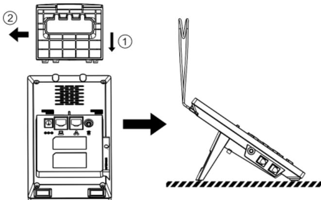
Figure 1 - Bracket installation
