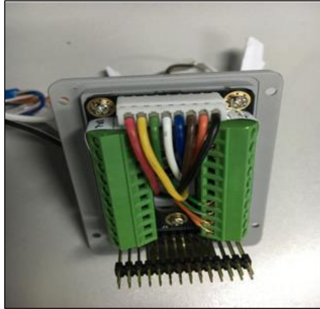
Figure 69: Wiegand Interface Cable
