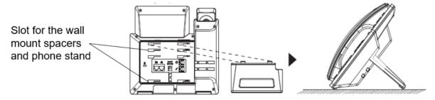
Figure 2: phone Stand and Mounting Slots on the GRP26XX
