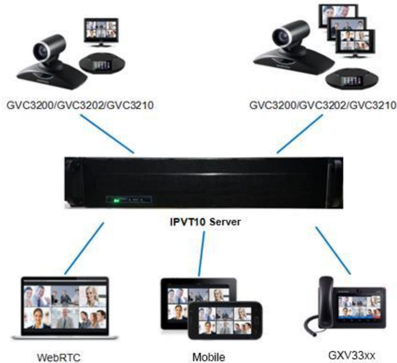
Figure 1: IPVT10 Video Conferencing System Architecture
