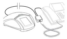
Unplug the telephone handset cable from the phone and connect it to the adapter as illustrated above.
