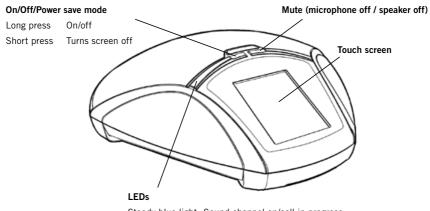
Steady blue light Sound channel on/call in progress Steady red light Mute, microphone turned off
