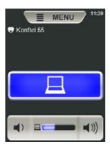
The computer normally only activates the speaker in the Konftel 55 if there is no other program running that can use the microphone. This means that the Konftel 55 acts as a computer speaker and that the audio processing in OmniSound® HD is turned off so that the sound is not altered.
