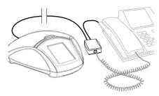
Unplug the telephone handset cable from the phone and connect it to the adapter as illustrated above.
