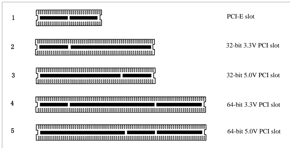
Figure 2 PCI-E and PCI slots
