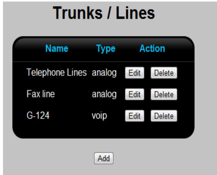
Analog lines are used to connect to the traditional PSTN (Public Switched Telephone Network). G-Series Gateway units with FXO ports offer Kewl Start or Loop Start. They can accommodate up to four analog lines. A single analog phone set can be connected to each available FXS port.
