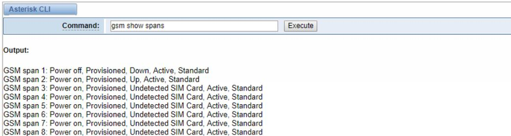
The screenshot shows a web interface for the Asterisk CLI. At the top, there is a tab labeled "Asterisk CLI". Below the tab, there is a "Command:" label followed by a text input field containing "gsm show spans" and an "Execute" button. Below the command field, there is an "Output:" label followed by a list of GSM span status information:
