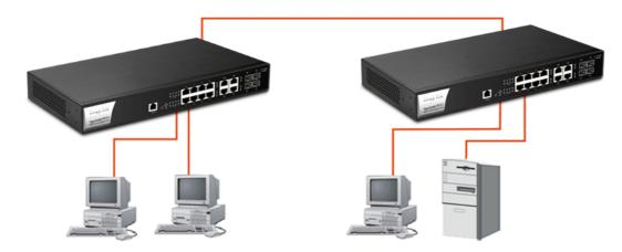
If VLAN is enabled and configured, each node in the network that can communicate each other directly is bounded in the same VLAN area.
