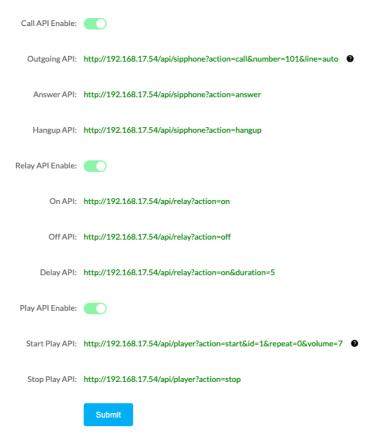
(Note: Authentication and encryption are not used in the API interface, so please pay attention the security of the network environment when opening and using these API interfaces).
