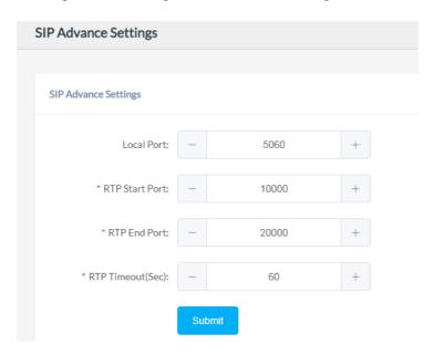
• Local Port: This setting represents the port that used to received SIP packets.
