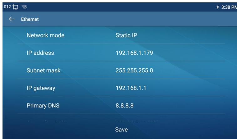
*Picture 107 - Static IP network mode*
