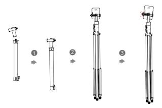
Position the thread of the base station clip on the stand and screw the base station clip into place.
