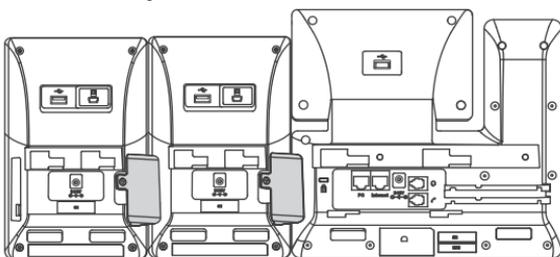
Note: The T52S/T54S/T56A/T58A/T58V IP phone can support 3 expansion modules at most. But if you use more than one expansion module, you need to connect an additional Yealink power adapter (5V/2A) to any one of the expansion modules. The power adapter should be purchased separately.
