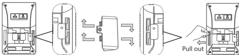
The slots are plugged up by silica gel. You can pull out the silica gel when cascading expansion modules.
