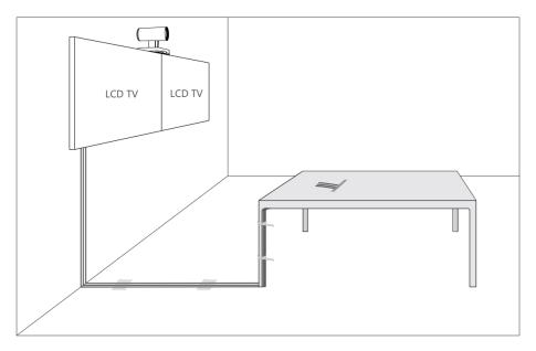
Note: If the cable length exceeds 7 meters, USB extension cables can be used for wiring.
