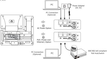
Note: The IP phone should be used with Yealink original power adapter (5V/2A) only. The use of the third-party power adapter may cause the damage to the phone. If you are connecting a PC to your phone, we recommend that you use the Ethernet cable provided by Yealink.
