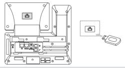
Note: The USB port can also be used to connect the Wi-Fi USB dongle WF40, color-screen expansion module EXP50 and USB headset.
