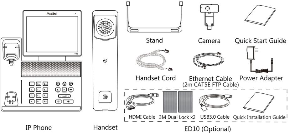
Note: The Extended Display Accessories ED10 helps you display the video image captured from the camera (both near site and far site) on the external monitor during a video call. For more information, refer to Yealink Extended Display Accessories Quick Installation Guide for SIP VP-T49G. We recommend that you use the accessories provided or approved by Yealink. The use of unapproved third-party accessories may result in reduced performance.
