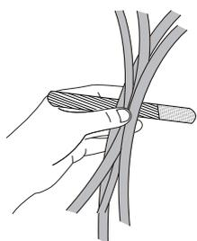
Fasten the cables with the cable tie
