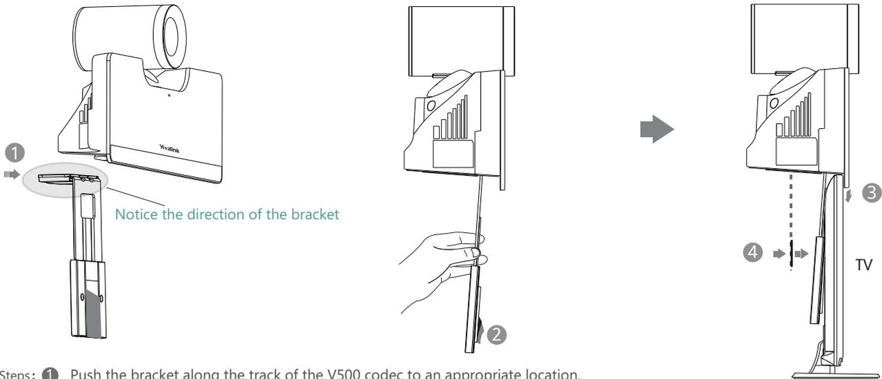
Steps: ① Push the bracket along the track of the V500 codec to an appropriate location.
