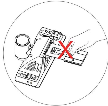
💡 If your VC500 codec cannot be mounted on the top of a TV when the bracket has reached the edge of the VC500 codec, choose other installation methods. The VC500 codec may fall down when the thickness of the TV is more than 77 mm. In this situation, do not mount the VC500 on the top of a TV.
