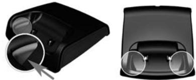
You can also remove the guides by pressing a suitable screwdriver in the longish holes on the bottom of the charger.
