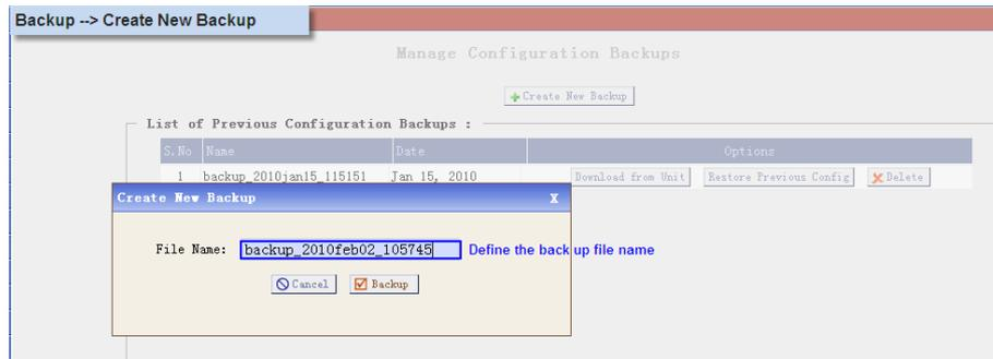
After the back up, you can see the back up in the back up file list. you can restore the configure in this page also. Note that the restore will only work after reboot.
