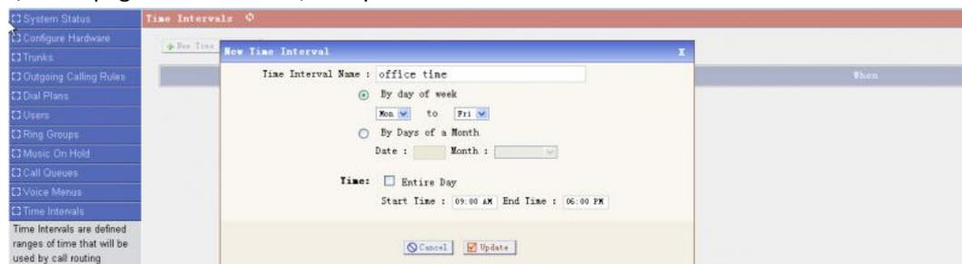
2/In the page **Incoming Calling Rule**, set up the rule with time Interval, then the incoming calls will be routed to the corresponding destination during these hours.
