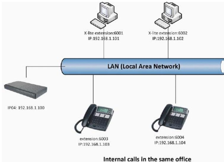
At the beginning, we need to add some extensions to make internal calls. Each extension acts as an internal number. There are three types of extensions we can add: SIP, IAX2 and ZAP.
