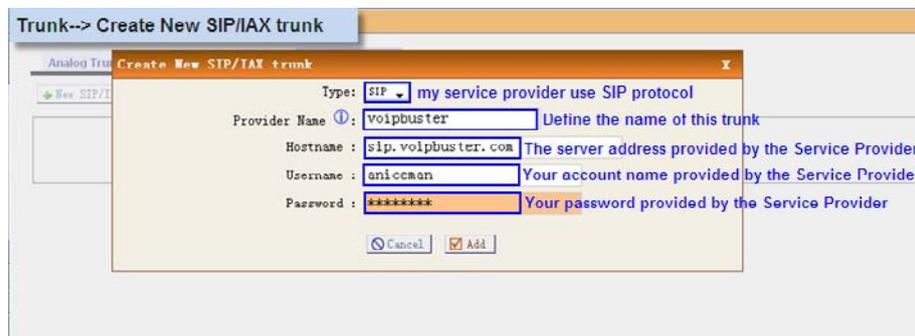
There are many service provider provide voip calls. Any provider use standard Sip or IAX2 protocol should work with the IP-PBX
