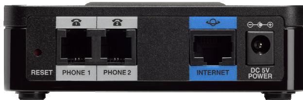
Figure 2. Ports on Cisco SPA112 ATA 2 Port Adapter
