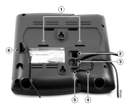
STEP 1 Turn the phone body over to expose the ports on the back of the unit.
