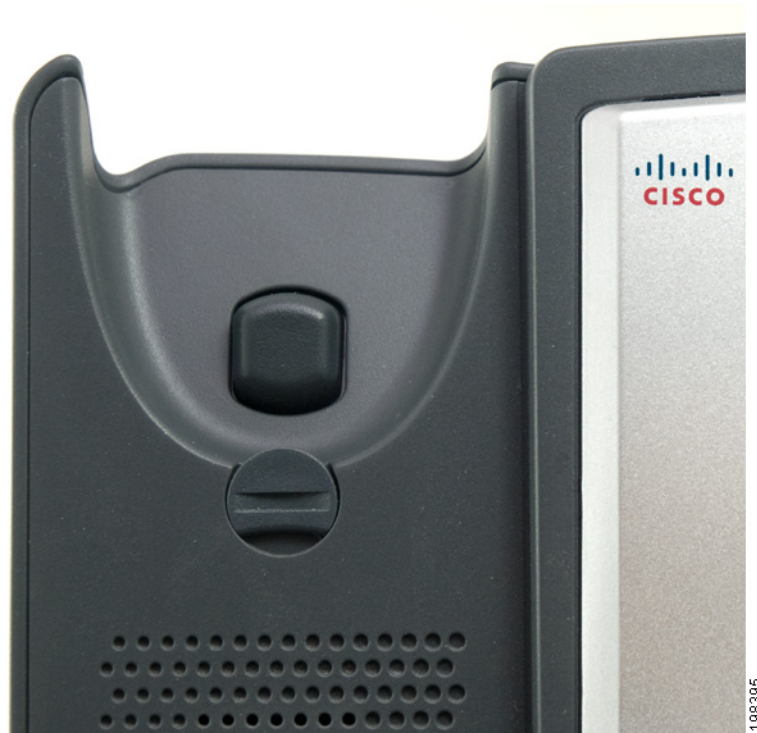
Figure 6 Handset Retention Tab (Reversed)
