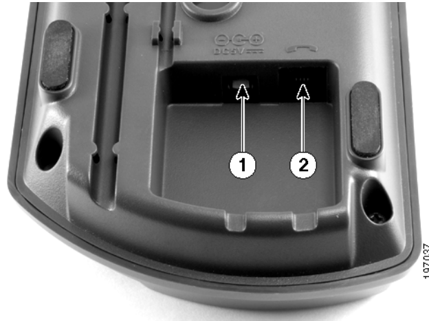
Figure 1 Cisco SPA 301 Phone Power and Handset Connections
