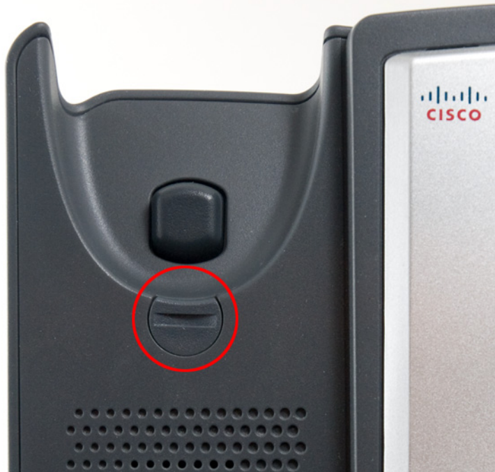
Figure 5 Handset Retention Tab (Default Position)
