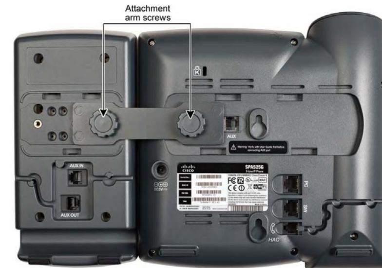
**CAUTION** Do not plug a telephone line cord into the AUX port. Use only the auxiliary cable provided with the SPA500S.
