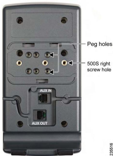
**STEP 7** Using an attachment arm screw, secure the attachment arm to the Cisco SPA 500S.
