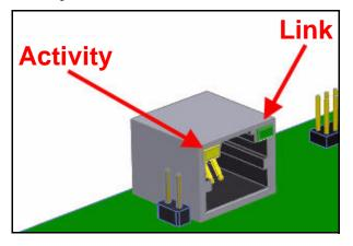
3.2. The **GREEN Link** LED blinks off once during the boot up process and then comes on again and remains constant (solid **GREEN**). The **YELLOW Activity** LED may be blinking depending on the network activity.
