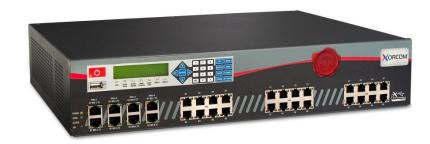
provided by connecting up to 24 external <u>Astribank</u> units via the USB2 ports, for a total of up to 800 PSTN/analog phones ports, up to 1000 users and up to 480 concurrent calls.
