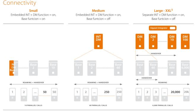
One Hardware for all functions: N870IP appliance. Function is set in the device settings: Integrator, DECT Manager and/or Base station. 5 In preparation, available at a later point in time
