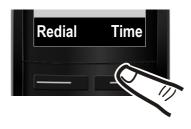
Press the key below Time on the display screen to open the input field.
