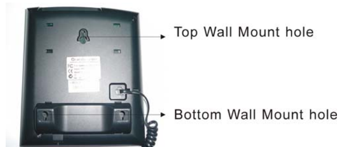
Figure 3: Location of the fixed hanger on GXP280
