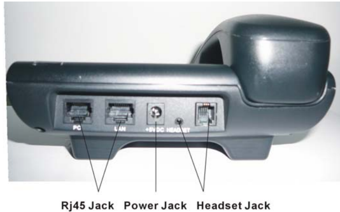
Figure 1: Connectors on the back of the GXP280
