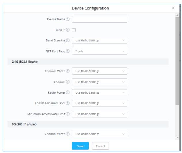
Figure 56: Access Point Configuration Page
