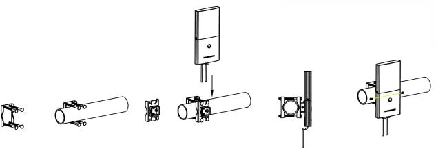
Figure 17: GWN7600LR Horizontal Mounting
