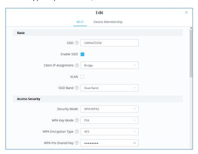
Figure 59: Add a new SSID
