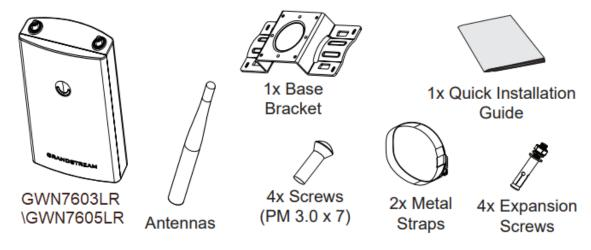
Figure 3: GWN7630LR/GWN7605LR Equipment Package
