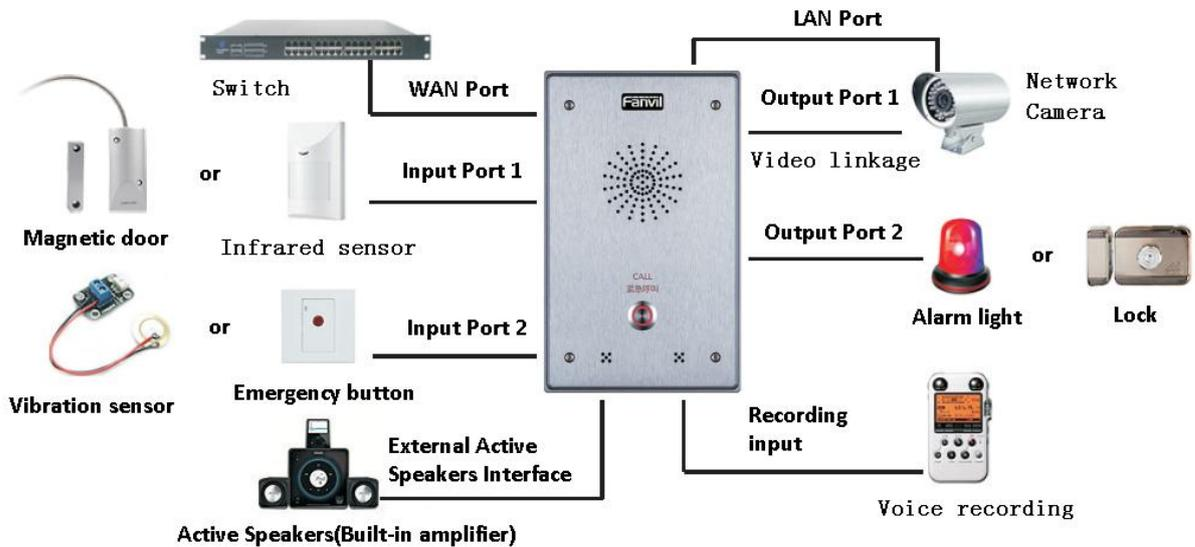
Figure 1 - Connection Diagram
