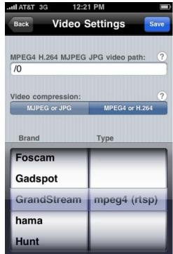
The video path shown in the picture above, represents the port where the application will be listening at. When selecting 'Grandstream' from the brand list, it will automatically select /0, this means that it will be listening the **primary stream** of port one. If you want to listen to the secondary stream of same port one, then you can select /4 For more information about the port and channels please see the description for the MJPEG below.
