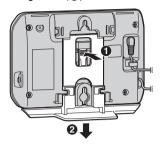
2 Mount the base unit by inserting the screws (not supplied) into the round openings on the unit, then slide the unit down to secure it.
